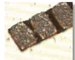
2D+3D Image with clear low bridge defect
