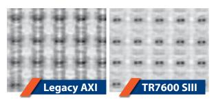
TR7600 SIII delivers improved 3D image quality for shielded components and high-density connectors
