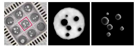
Solder voiding inspection and analysis using 3D and CT images
