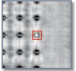
Press Fit Pin Defect
