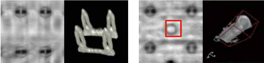
3D CT displays solder joints and defects in much more detail than traditional 3D X-ray slicing
