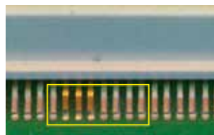
Lifted leads clearly identified using angle view camera.
