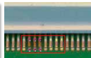
Lifted leads clearly identified using angle view camera.
